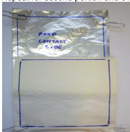
3) Repeat for second portion and overlay 4) Heat seal together to form pouch
