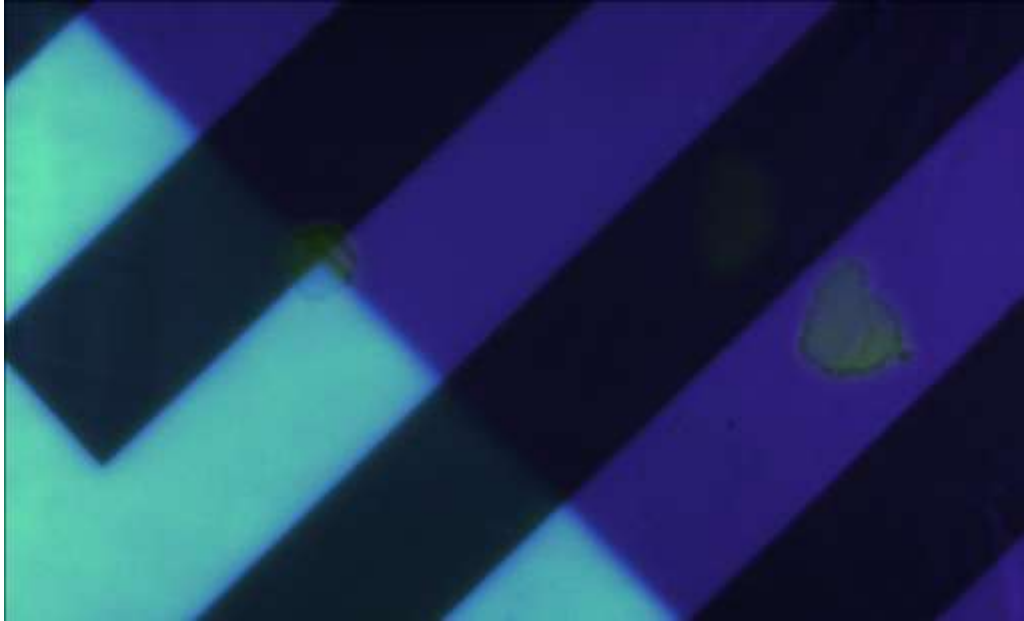
Figure 26 - Thin white film (with print show-through) contaminated with IRGACURE 379 under UV illumination
