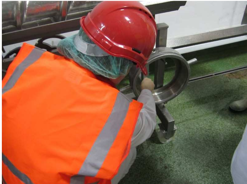
Experiment 1 – Swab 12– Repeat swab after locking screw re-cleaned.
