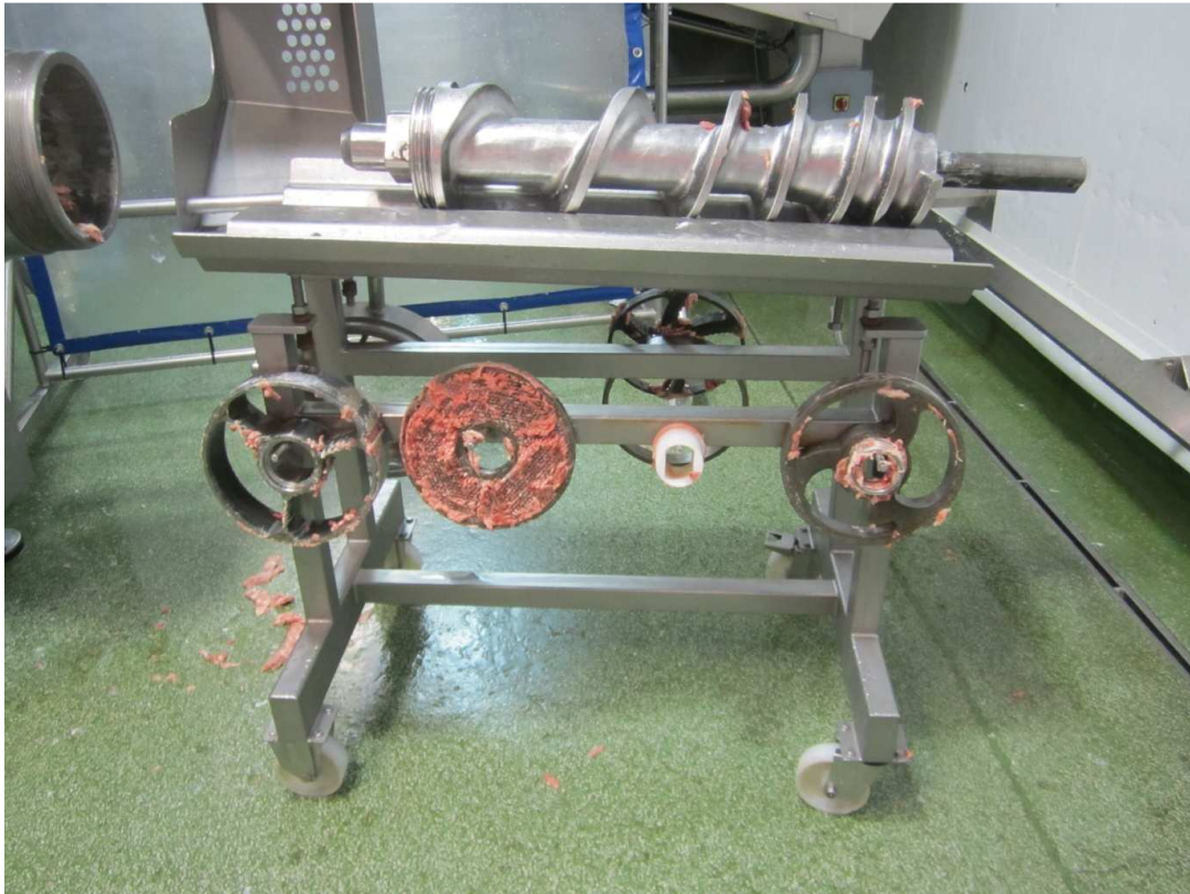
Photograph 1 – Grinder dismantled and ready for cleaning
